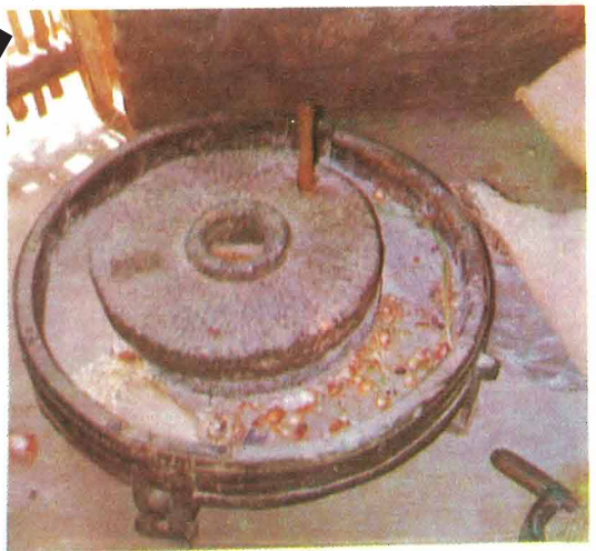
Photo 13. 'Chakki' - a local grain grinding machine used by tribal women.
